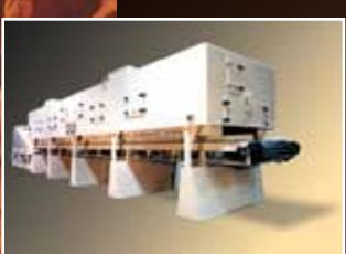
*Wolverine Proctor Dryers are used throughout the tobacco industry to dry, toast, cool, expand and reorder tobacco in all stages of its processing from the threshing plant to the final manufactured product.*
